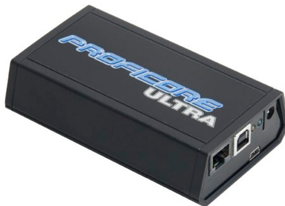
ProfiTrace 2 firmy gridconnect to analizator sieci fieldbus.
